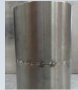
Pipe butt weld Ø 31.75 x 2 mm
